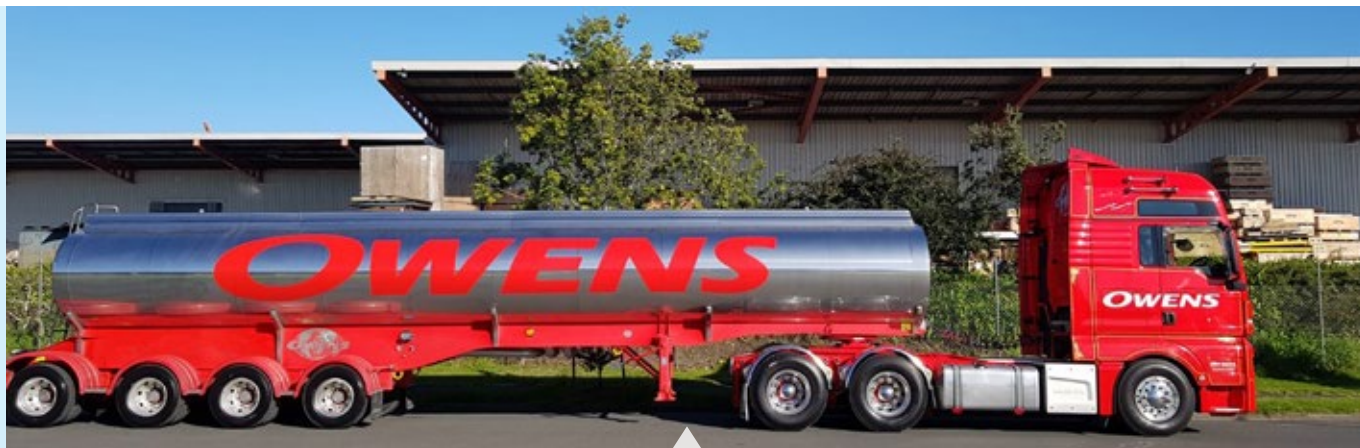
The new Owens quad-axle tanker capable of 32,000 litres (4 x 8,000 litre compartments), dedicated Auckland to Wellington return
